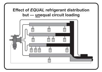
These illustrations depict conditions that result in a loss of heat transfer due to either (top) unequal circuit loading or (bottom) unequal refrigerant distribution.
